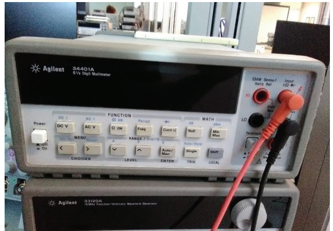
FIGURE 2. Agilent 34401A multimeter used to measure AC voltage
