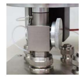
carousel to add samples it is only necessary to turn the valve, isolating the entire carousel section. The carrier gas will continue to flow through the rest of the analytical circuit. After adding samples to the carousel, close the lid, turn on the purge flow and let the carousel purge for 2-5 minutes. Close the purge vent, turn off the purge flow, and open the isolation valve.
